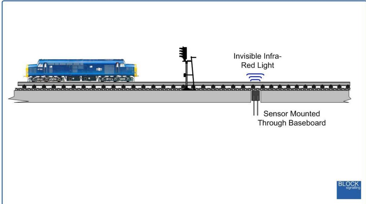
The detector can be mounted in an 8mm hole drilled through the track baseboard. If required, the detector can be held in place using a small amount of blutack, expanded polystyrene or similar.
