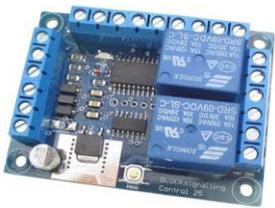
The SAS1 can operate 2-aspect signals at the end of the line and provides variable or random delays in either direction.
