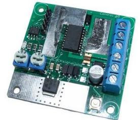
You don't need a separate DC controller with the SS2A, as it has one built-in. Just connect a 12V DC power supply.
