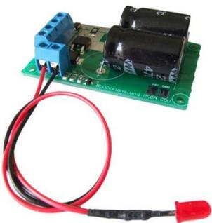
The CDU2RL has a built-in led which illuminates when the capacitors are charged to 15V or above. This can be panel mounted.
