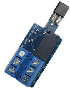
The BOD2-RLY has a built-in changeover relay which operates when a train passes over the infra-red sensor. Works in tunnels.
