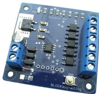
The TLC1A is for common-cathode (common-negative) traffic light signals.
