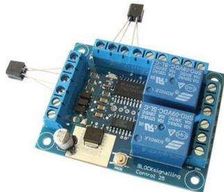
The SAS2-IR uses infrared sensors to detect the train arriving at the end of the line. No track breaks are required.
