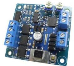
For DCC users, the SDCC1 provides shuttle operation and stations stops, with speed and waiting time adjustable.
