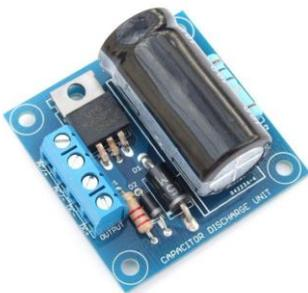
The CDU1C is suitable for smaller layouts where points are operated individually.
